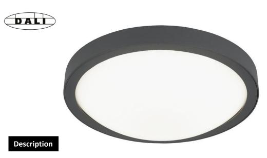
Surface mounted, round LED fitting with increased ingress protection class IP65 and integrated energy-saving LED light source. Body and base made of high-pressure cast aluminium and powder coated silver or graphite. Specially formed diffuser made of impact resistant PC ensures the highest possible impact resistance of the fitting (IK10). Color temperature 3000K/4000K, CRI>80, SDCM  $\leq$  3,
